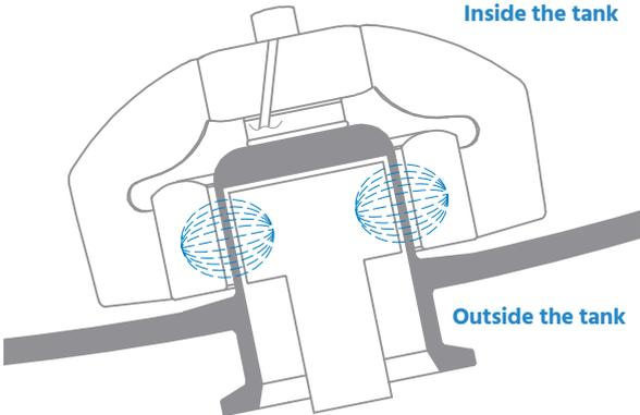
The Drive Unit connects to the Mixing head magnetically from the outside through the stainless steel of the tank plate.
