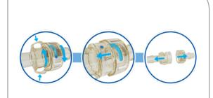
To disconnect two MPU components, depress the two latches on the insert (or plug) component while twisting the two separate MPU components ¼ turn to separate.
