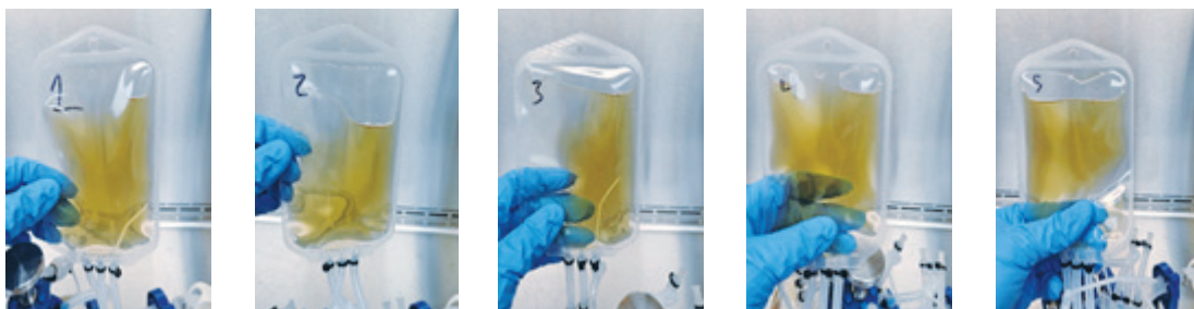
FIGURE 1: SAMPLE BAGS CONTAIN CLEAR NON-TURBID MEDIA AFTER INCUBATION AT 37°C FOR 72 HOURS
